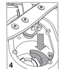
After cleaning the filters, re-place the filter assembly and fix it in position correctly; this is essential for maintaining the efficient operation of the dishwasher.
