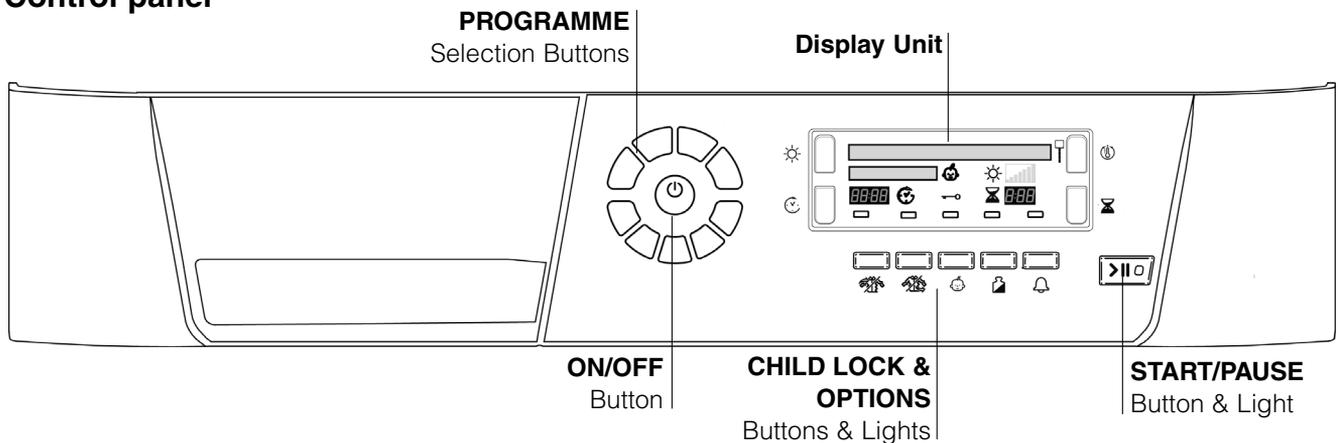
The **ON/OFF** button - if pressed when the dryer is running: If the display shows **TURNING OFF** the dryer stops. If the display shows **PRESS AND HOLD** hold the button and the display counts down 3, 2, 1 and then stops. Press and hold again for more than 3 seconds, the display briefly shows **POWER ON**.
