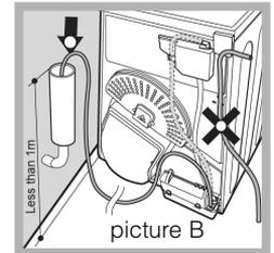
Then fit a suitable length of hose to position shown in picture B.
