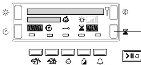
After selecting a programme that has a Timed Dry option, press the ⌚ Timed button and the display will increment the selected time, each time you press and release the button (see *Start and Programmes*).
