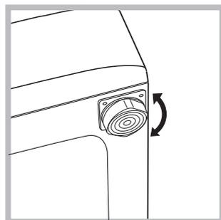
1. Install the washer-dryer on a flat sturdy floor, without resting it up against walls, cabinets or anything else.
