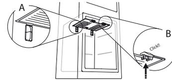
7. Reinsert the upper drawer and close the door of the freezer compartment.
