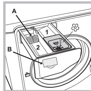
! Do not pour detergent into the compartment 1. Detergent should only be poured into the compartment 2.
